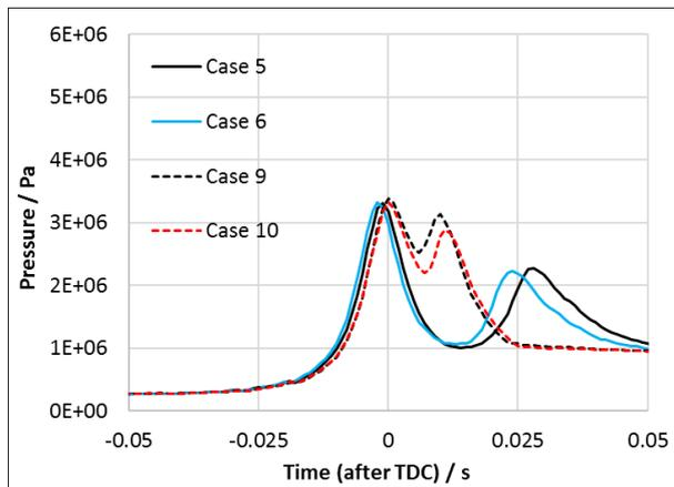
Fig. 6. Pressure traces for setup without prechamber; Cases 5-6 – methane, Cases 9-10 – ethane.
