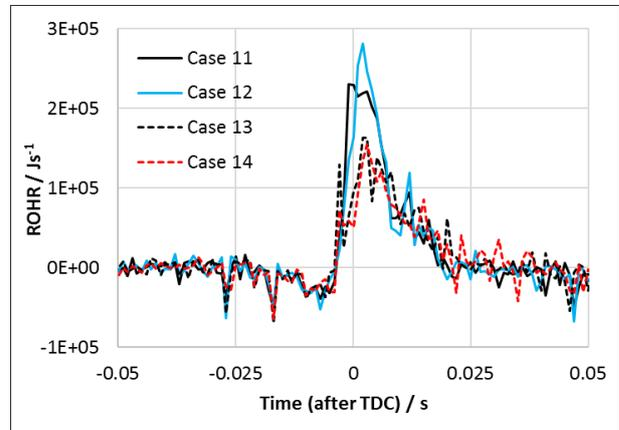
Fig. 11. ROHR for lean mixtures for setup with prechamber; Cases 11-12 – methane, Cases 13-14 – ethane.
