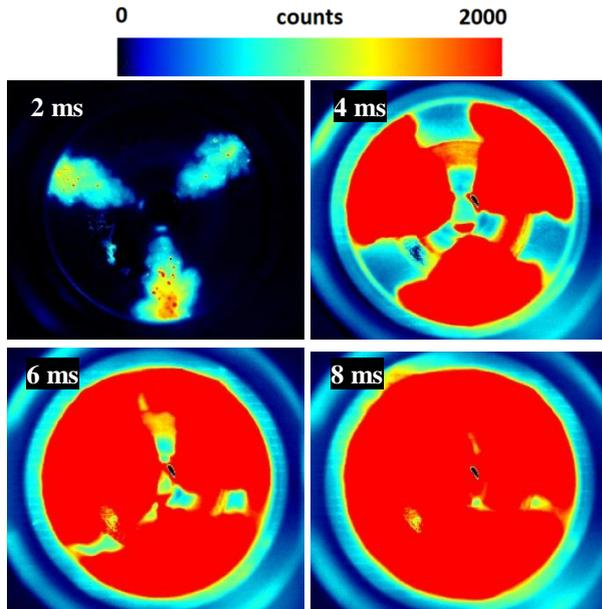
Fig. 5. Visualised flame for Case 4; images taken 2, 4, 6 and 8 ms after ignition.
