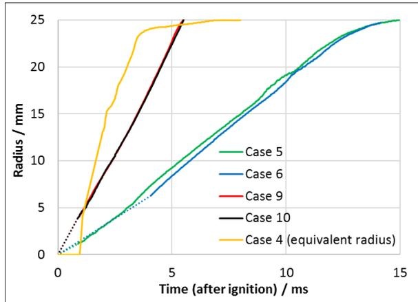
Fig. 9. Flame radius evolution; Cases 5, 6, 9 and 10 – flat head, Case 4 – prechamber (equivalent radius).
