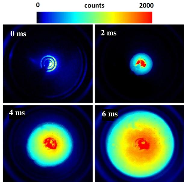
Fig. 8. Visualised flame for Case 2; images taken 2, 4, 6 and 8 ms after ignition.
