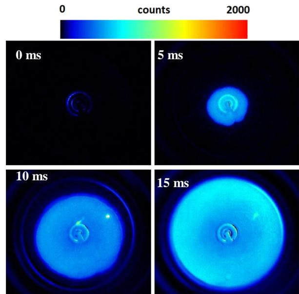
Fig. 4. Visualised flame for Case 6 at instance of ignition and 5, 10 and 15 ms after ignition.
