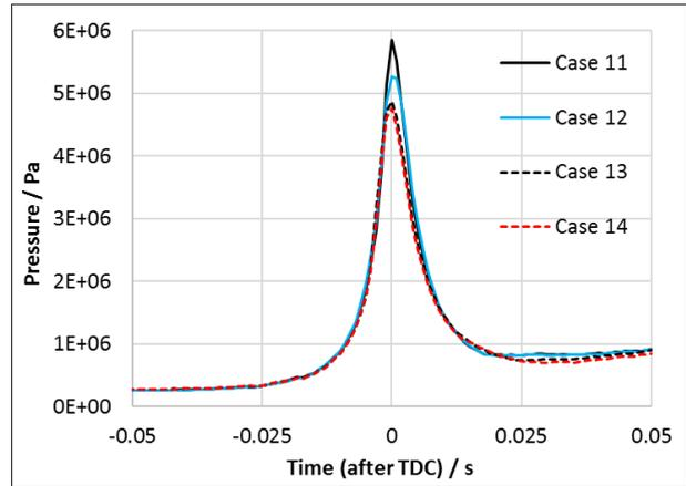
Fig. 10. Pressure traces for lean mixtures for setup with prechamber; Cases 11-12 – methane, Cases 13-14 – ethane.
