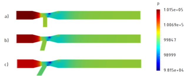
**Fig. 11.** Contours of pressure loss between analysed cases – a)  $0^\circ$ , b)  $15^\circ$  and c)  $30^\circ$  [Pa].
