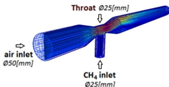
Fig. 1. Venturi mixer design with dimensions [mm].
