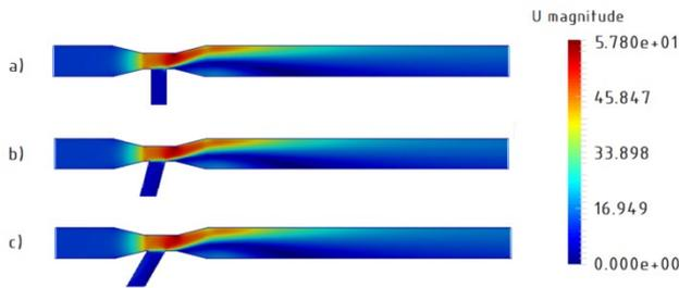
**Fig. 9.** Contours of velocity magnitude between analysed cases – a)  $0^\circ$ , b)  $15^\circ$  and c)  $30^\circ$  [m/s].
