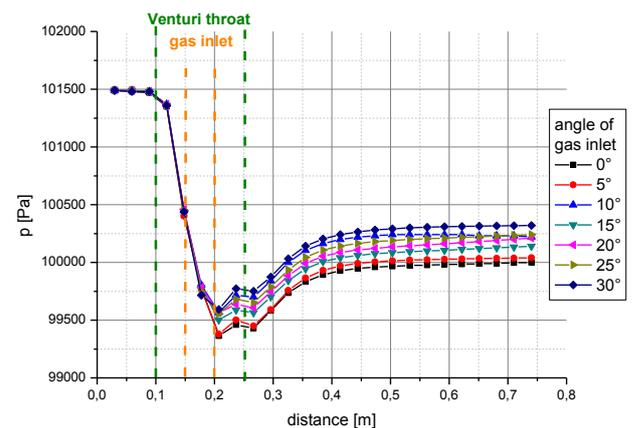
**Fig. 12.** Pressure loss [Pa] through the Venturi mixer for different gas inlet angles.
