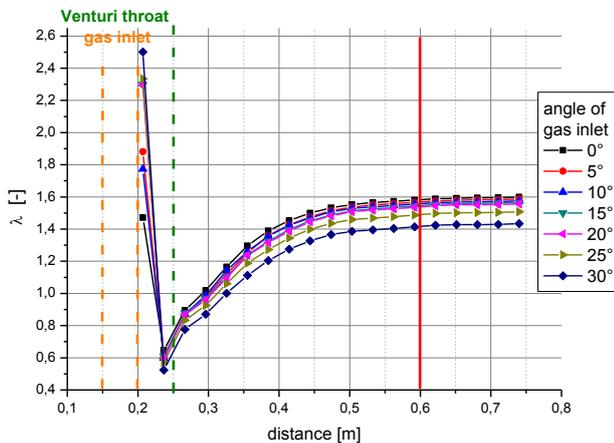
**Fig. 7.** Distribution of air excess coefficient  $\rightarrow \lambda$ , through the Venturi mixer for different gas inlet angles.
