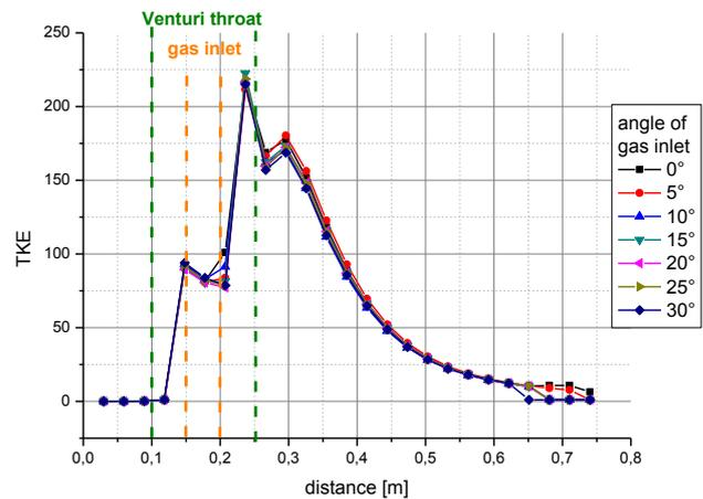
**Fig. 8.** Distribution of Turbulent Kinetic Energy (TKE) through the Venturi mixer for different gas inlet angles.
