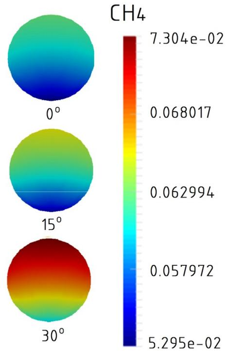
Fig. 4. Distribution of methane mass fraction in the cross-sectional view between analysed cases – 0°, 15, 30° at the outlet of the Venturi mixer at 0.74 [m] from the inlet.
