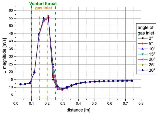
**Fig. 10.** Distribution of velocity magnitude [m/s] through the Venturi mixer for different gas inlet angles.
