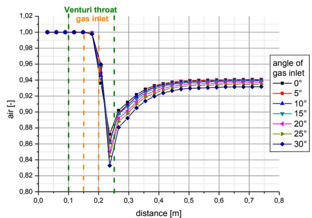
**Fig. 6.** Concentration of air through the Venturi mixer for different gas inlet angles.
