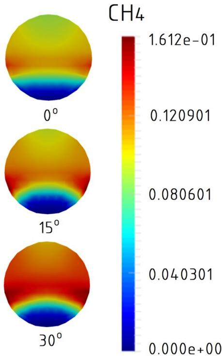
Fig. 3. Distribution of methane mass fraction in the cross-sectional view between analysed cases – 0°, 15, 30° after passing the Venturi throat at 0.25 [m] from the inlet.
