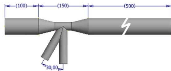
Fig. 2. Analysed cases (0°-30°) with the dimensions [mm].
