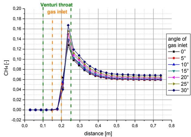
**Fig. 5.** Concentration of methane mass fraction CH<sub>4</sub> through the Venturi mixer for different gas inlet angles.
