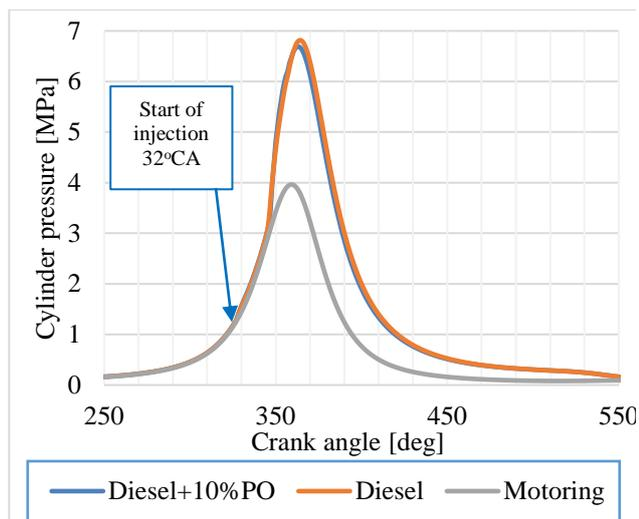
Fig. 7. Cylinder pressure vs. crank angle range 250÷550 deg for a variable fuel
