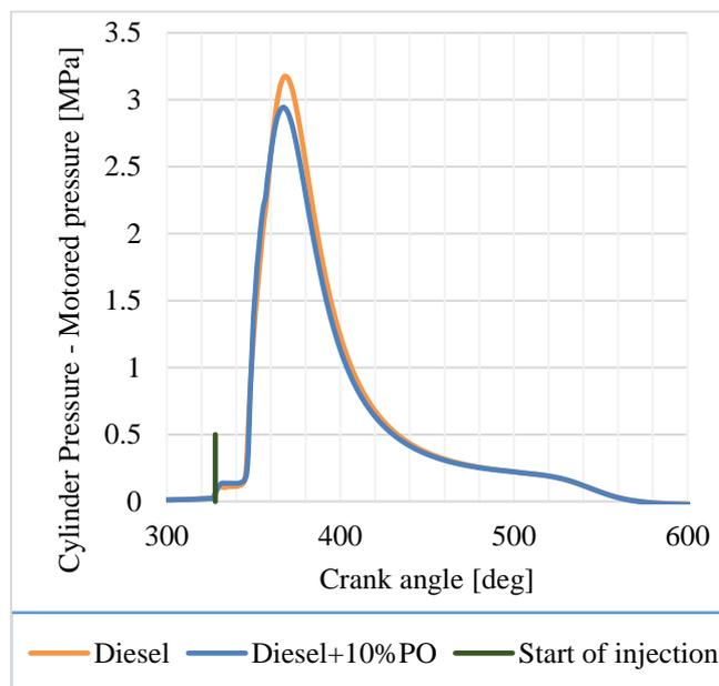
Fig. 10. Pressure increase as a result of fuel combustion
