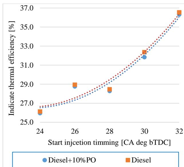
Fig. 12. Indicated thermal efficiency curves
