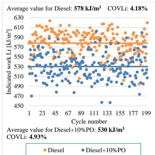
Fig. 8. Unrepeatability of the engine work for reference fuel and for research fuel
