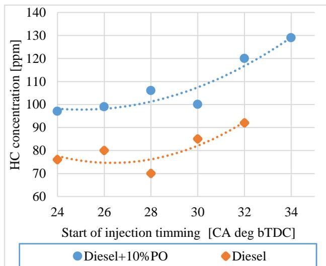
Fig. 15. HC concentration in exhaust gases
