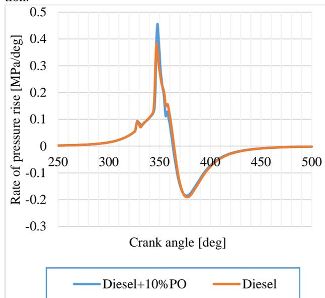
Fig. 9. Rate of pressure rise vs. crank angle
