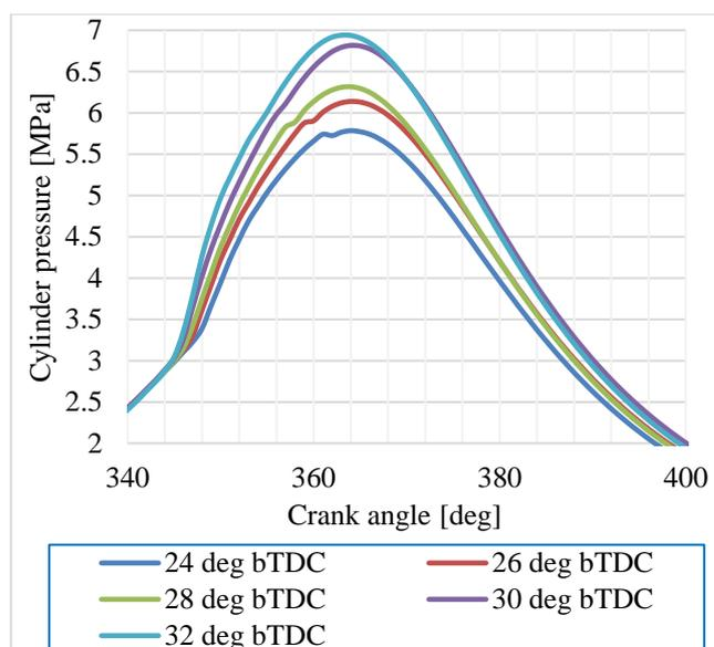
Fig. 5. Cylinder pressure vs. crank angle range  $340\div 400$  deg for a variable start of fuel injection, fuel: Diesel
