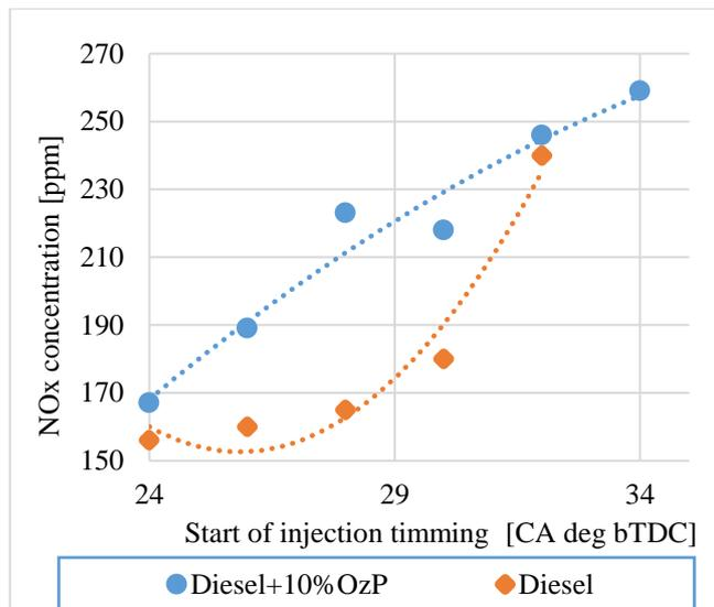
Fig. 14. NOx concentration in flue gases
