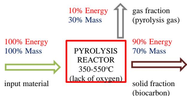
Fig. 1. Exemplary mass and energy distribution in pyrolysis process
