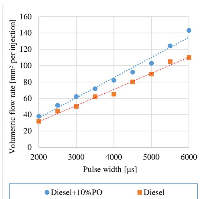
Fig. 11. Characteristic curves of the injection rate for both fuel
