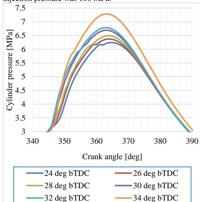
Fig. 6. Cylinder pressure vs. crank angle range  $340\div 390$  deg for a variable start of fuel injection, fuel: Diesel+10%PO
