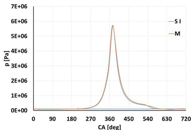
Fig. 1. Pressure trace comparison between test engine and simulated model
