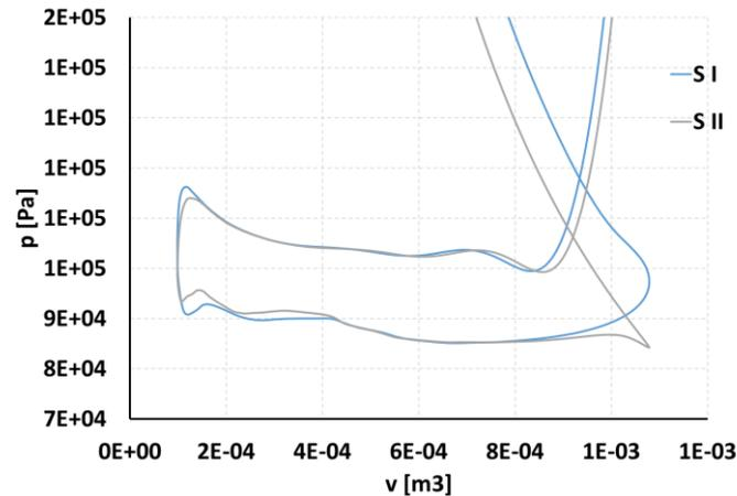
Fig. 4. Comparison of charge exchange loop pressure trace for engine with configuration S I and S II
