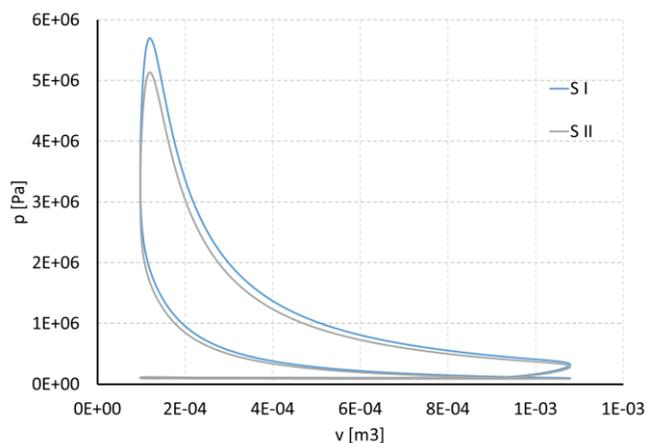
Fig. 3. Comparison of pressure trace for engine with configuration S I and S II
