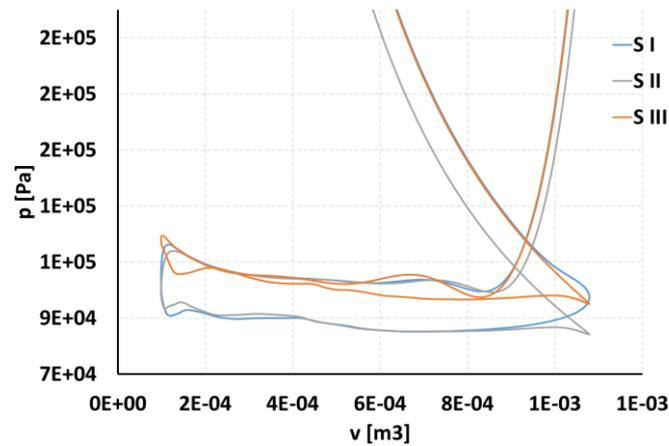
Fig. 5. Comparison of charge exchange loop for three simulated cases
